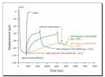
Fig. 7**B**. Expansion of dried demineralized dentin matrix by various ethanol/HEMA concentrations, with values in  $(J/cm^3)^{1/2}$  given in parentheses. Note that 30% ethanol/70% HEMA at a  $\delta_n = 16.7$  could not expand the matrix, but that 50% ethanol/50% HEMA at a  $\delta_n$  of 17.6 could slowly expand the matrix.
