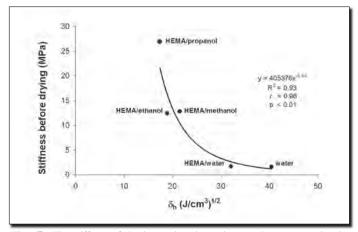
Fig. 4**D**. The stiffness of dentin matrices just prior to solvent evaporation is compared to the Hoy's solubility parameter for hydrogen bonding ( $\delta_h$ ) of water and 35% HEMA/65% alcohol mixtures. Note that the  $\delta_h$  values for primers needs to be about 20 (J/cm<sup>3</sup>)<sup>1/2</sup> to develop significant matrix stiffness (from Eddleston *et al*,<sup>11</sup> with permission).
