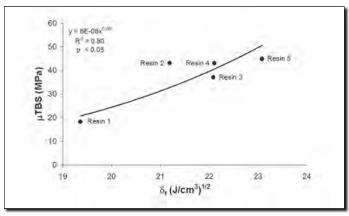
Fig. 9**B.** Comparison of microtensile bond strengths ( $\mu$ TBS) of five experimental resins described in Table 5 as a function of their hydrophilicity ranked by their Hoy's solubility parameter for total cohesive forces ( $\delta_t$ ) when 50 wt% ethanol was applied to acid-etched, ethanol-saturated dentin. Note that all bond strengths except resin 5 were higher than those shown in Fig. 9A and resin 2, a very hydrophobic resin, gave high bond strengths.
