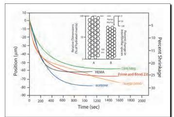
Fig. 7A. Shrinkage of water-saturated demineralized dentin matrix in response to 100% acetone, 100% HEMA, Prime & Bond 2.0.<sup>c</sup> One-Step<sup>d</sup> or Single Bond.<sup>e</sup> All treatments caused a 20-25% shrinkage of the matrix due to water loss from the matrix into the excess solutions. Insert shows schematic of how intertubular dentin could shrink by loss of interfibrillar spaces rather than any change in fibril diameter.
