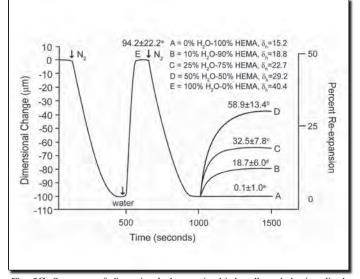
Fig. 3C. Summary of dimensional changes in dried, collapsed demineralized matrix that was 200  $\mu$ m thick in response to A = 100% HEMA (no expansion), B = 10% H<sub>2</sub>O/90% HEMA (slow 19% expansion), C = 25% H<sub>2</sub>O/75% HEMA (faster, 33% expansion), D = 50% H<sub>2</sub>O/50% HEMA (relatively rapid, 59% expansion).
