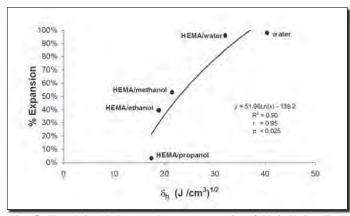
Fig. 4**B.** The relationship between the percent expansion of dried, demineralized dentin and the Hoy's solubility parameter for hydrogen bonding ( $\delta_h$ ) of water and HEMA/alcohol primers. Note that 35% HEMA/propanol ( $\delta_h = 16.2$ ) could not expand the matrix, while HEMA/ethanol ( $\delta_h = 18.3$ ) and HEMA/methanol ( $\delta_h = 20.9$ ) could partially expand the matrix (from Eddleston *et al*,<sup>11</sup> with permission).
