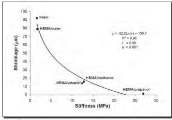
Fig. 4C. Plot of matrix shrinkage upon solvent evaporation *versus* the preevaporation stiffness of the matrix. Water and HEMA/water mixtures prevented interpeptide H-bonding, making the matrix too compliant to resist shrinkage. HEMA/ethanol and HEMA/methanol could not prevent all interpeptide H-bonds from forming, allowing a stiffness of the matrix of 12-13 MPa. This reduced the matrix shrinkage during solvent evaporation to only 16.18% (from Eddleston *et al*,<sup>11</sup> with permission).
