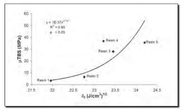
Fig. 9A. Comparison of microtensile bond strengths ( $\mu$ TBS) of five experimental resins described in Table 4 as a function of their hydrophilicity ranked by their Hoy's solubility parameter for total cohesive forces ( $\delta_1$ ) when 50 wt% ethanol/50% resin mixtures were applied to acid-etched, water-saturated dentin.
